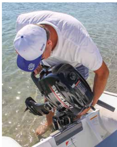
Right: Simple screw clamps make mounting and removal a breeze.
